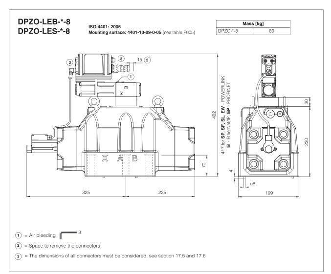
Notes: the overall height is increased by 40 mm for /G option (0,9 kg); for option /B the proportional solenoid, the LVDT transducer and the on-board digital driver are at side of port B of the main stage
