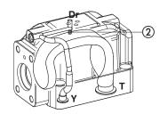
Internal piloting: Without blinded plug SP-X500F ①; External piloting: Add blinded plug SP-X500F ①; Without blinded plug SP-X300F ②; Internal drain: **External drain:** Add blinded plug SP-X300F ②.
