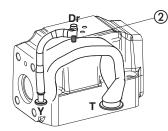
Internal piloting: Without blinded plug SP-X300F ①; External piloting: Add blinded plug SP-X300F ①; Internal drain: Without blinded plug SP-X300F ②; **External drain:** Add blinded plug SP-X300F ②.
