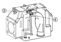
Internal piloting: Without plug ①; External piloting: Add NPTF 1/8 in pos 1);
