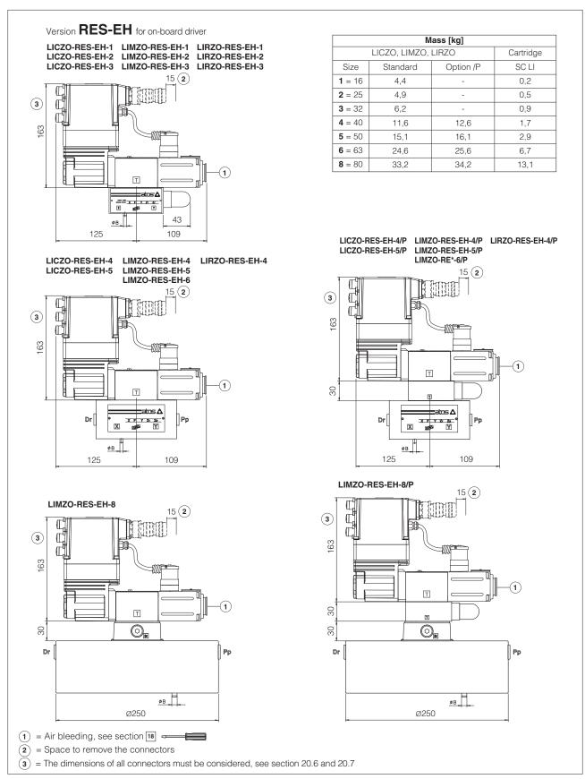
Note: for mounting surface and cavity dimensions, see tech. table P006
