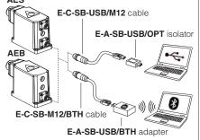
WARNING: drivers USB port is not isolated! For E-C-SB-USB/M12 cable, the use of isolator adapter is highly recommended for PC protection
