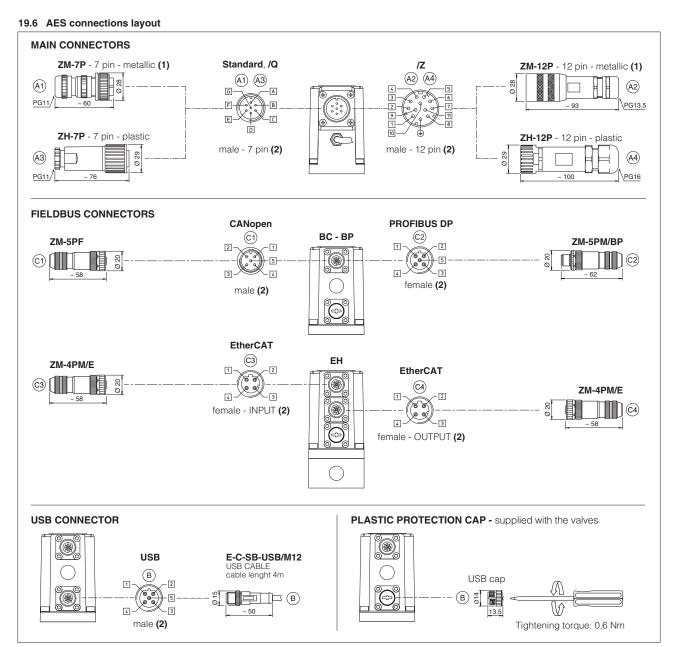
(1) Use of metallic connectors is strongly recommended in order to fulfill EMC requirements
