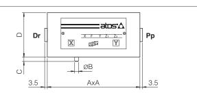
ze 1 cover is not squared but retangular, dimensions 65x80 ze 8 cover is not squared but circular, dimension Ø250
