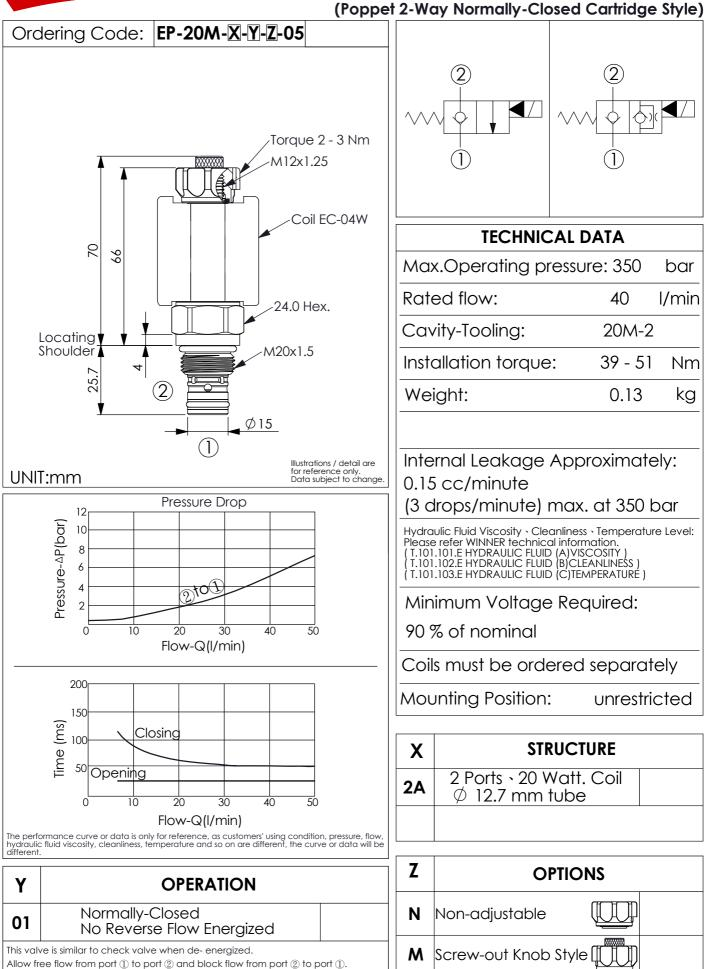
In energized condition, this valve is allowed flow from port (2) to port (1) but
