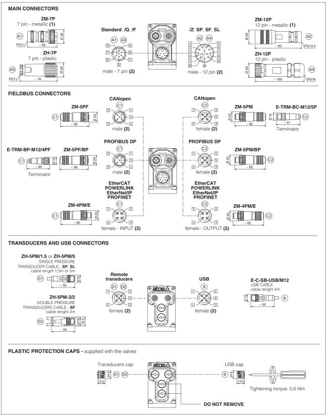
(1) Use of metallic connectors is strongly recommended in order to fulfill EMC requirements (2) Pin layout alw
