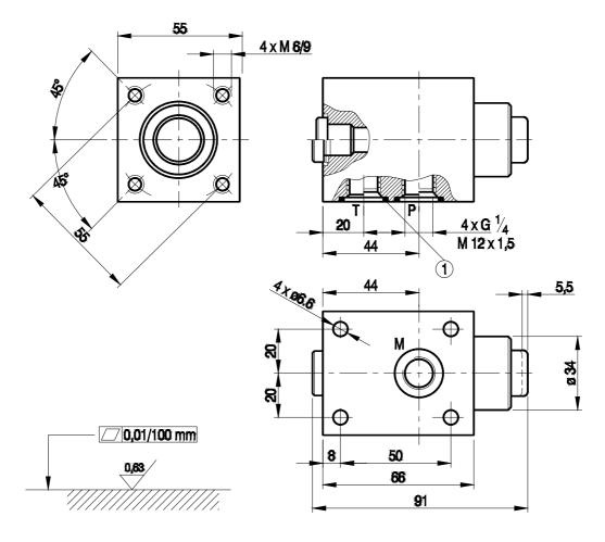
Admissible surface roughness and flatness deviation for a subplate face.
